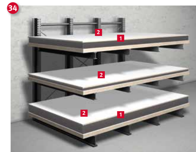
Horizontal storage of compact laminates
